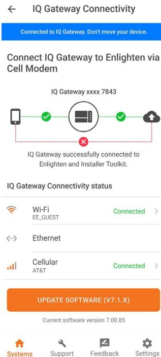
I. Repeat Step E through Step G to reconnect to the IQ Gateway. After rebooting the IQ Gateway, the Enphase Installer App takes approximately 10 minutes to display system metrics, including web connectivity, correctly. The gateway requires communicating with the web to display internet connectivity. For more information, contact [Enphase Support](#).
